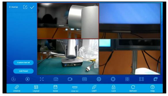
8. **PTZ**: On-screen PTZ control of the selected camera, including direction, zoom, focus, exposure, etc.
