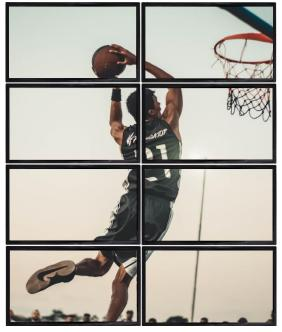
• Screen Splicing - This combines the selected screens into one and displays the selected input across all the splicing screens. For example, in the setup 2x4 at left, if all of them are spliced, then the input selected by the user will be displayed across all the 8 screens.
