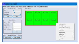
Once connected, G88 will load the settings used from last time. The default setting for the new unit out of package is 2x4 video wall with input 1 across the 8 screens. All outputs are set at resolution of 1920 x 1080@60.
