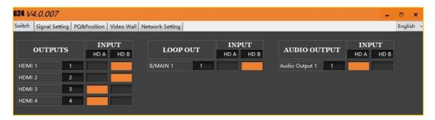
Users need to disable the video wall mode (Cancel the splicing) to enable the matrix switcher mode
