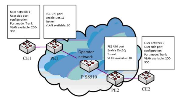
Figure 3 Typical configuration of Dot1Q tunnel
